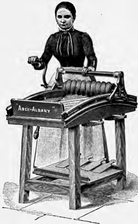
Fig. 64.—“Arch-Albany” Butter Worker, with Helical Roller.
